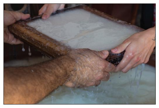
The paper making frame consists of a set of two frames. The bottom one contains a fine wire mesh, the top one forms the border for the paper.
