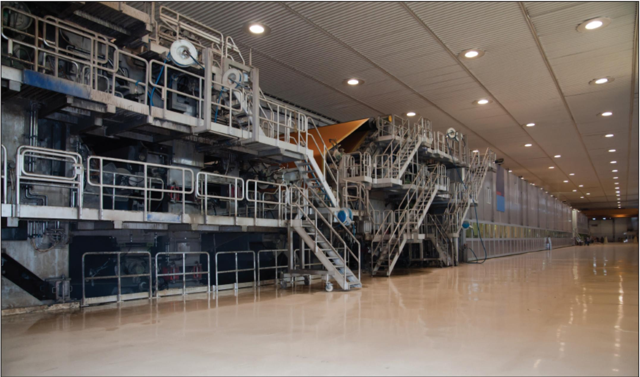
The wet pulp is sent through the paper making machine. The pulp enters the machine as a continuous stream. First, it is poured onto a on a wire mesh so that excess water can drain through. Then the paper moves through a series of pressing rollers and driers until it reaches the end of the machine.
